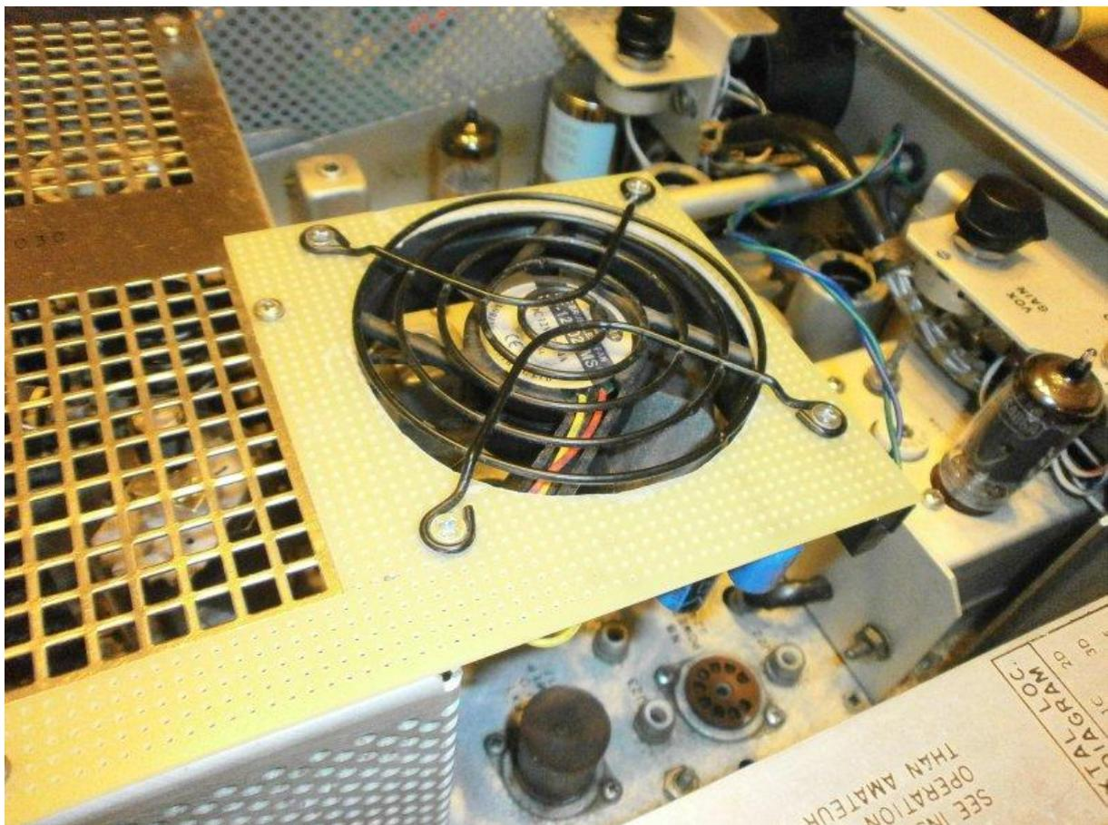
In the KWM-2/2A there is a lot of 6V AC (heaters, lamps), so I decided to built a AC-DC voltage doubler to feed the 12V DC fan. The circuit is very easy and small, built directly on the same PCB breadboard I used as fan bracket.
