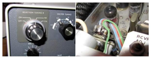
Here you can see the concentric former rejection tuning and power switch, and the RIT potentiometer mounted on the bracket that formerly held the variable capacitor.
