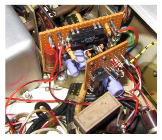
Actually, above you can see two boards. The one behind has the RIT components, and the one in front adds another function for CW: in transmit mode only, the PTO is shifted by the difference between the built-in sidetone frequency and the desired 800 Hz. That makes it possible to tune CW reception to 800 Hz and to be right on that frequency when transmitting.
