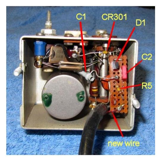
And my KWM-2 had a defective Waters rejection module. That had to move out and the tuning capacitor that was mounted concentric with the ON/OFF switch was replaced with a potentiometer for the variable bias voltage. As there is no noise blanker installed, the NB switch position can be used as RIT-ON. That even ensures that in CAL mode the RIT is always off.
