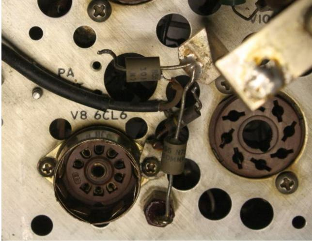
(13) Completely remove resistor R127 and capacitor C183. Proper unsoldering from that metal strip may need quite some heating power. Don't touch the other capacitor.
