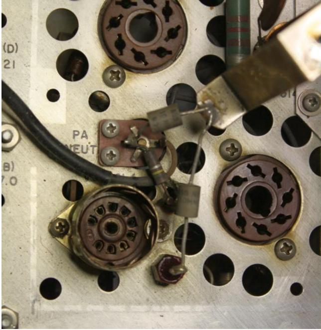
(12) Unsolder the inner conductor of the small piece of coax cable, the 100K resistor R127, and the 10 pF capacitor C183 from the small neutralizing capacitor C148. Then remove the two screws and capacitor C184. Now it should look like this:
